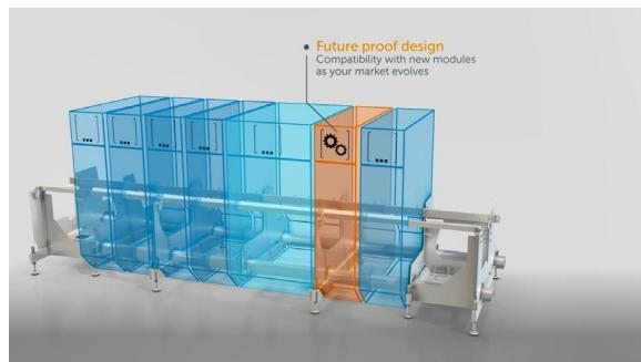
*Versatech is a future-proof filling solution, thanks in part to its standard-increment modules and centralized cabling network.*
