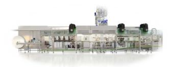
The Synerlink SL-FF 600 is a modular and evolutive form-fill-seal machine, forming up to 61,400 cups per hour.
