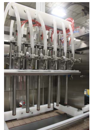
A close up of the CB50 six head inline filler.
