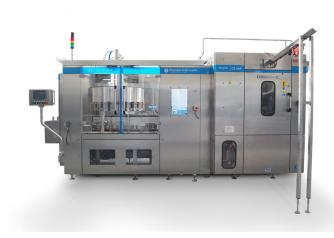
Pneumatic Scale Angelus' CB244 canning line, with integrated rotary filler and seamer, is capable of a variable speed range of up to 215 cans per minute.
