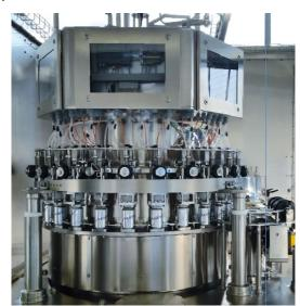
The integrated 24-valve rotary filler ensures flexible format changes and precise fill-level accuracy.
