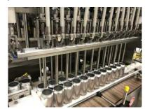
Pneumatic Scale Angelus' integrated 12-head inline filler ensures a perfect fill with little waste.
