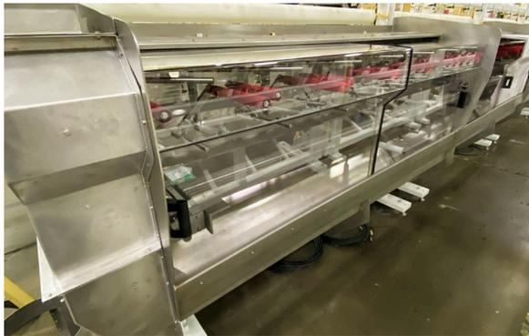
*Additional guarding, as seen on this Clipper currently in assembly, is one of the new design features on machines producing high-content alcohol wipes. It helps contain, control and extract/exhaust alcohol vapors.*
