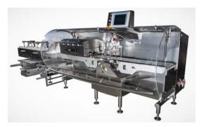
rounded legs to minimize debris build up and a 'No product - no bag' feature which minimizes film waste.
