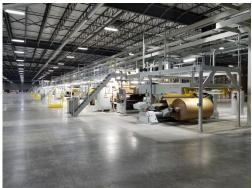
The new Maxco corrugator has a top speed of 1,300 feet per minute (400 meters per minute).
