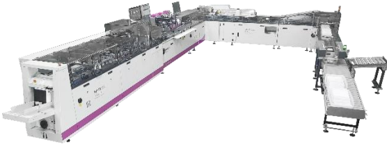
BW Converting's W+D BB820+ helps mail houses process more jobs in less time, running reliably at up to 20,000 cycles per hour.
