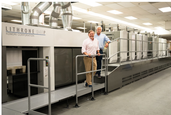
Kent and Tuck pictured by Tucker Castleberry's new Komori GL840P press, equipped with AMS Spectral UV LED-UV curing technology.
