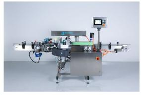
The Sirius 100, a cost-effective pressure-sensitive labeling machine, provides precise label placement accuracy for front, back and wrap applications in the personal care, household, food and pharmaceutical industries.
