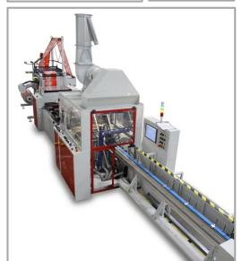
A recently developed product is the **EZ-Stand**, which provides the latest method for producing stand-up pouches (*pictured*, *top left*) by enabling traditional VFFS pouches to stand up! Innoflex, the creator of Inno-Lok® and Pour & Lok™, has developed new technology that pre-applies a bottom gusset to the film, which is then rolled up for later processing on a VFFS machine to create a stand-up pouch with only minor modifications to the sealing jaws.
