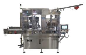
Pneumatic Scale Angelus' new CB100R counter-pressure canning line employs a 12-head rotary filling turret, coupled with a 3-spindle rotary seamer, to allow the machine to fill more than 100 CPM.
