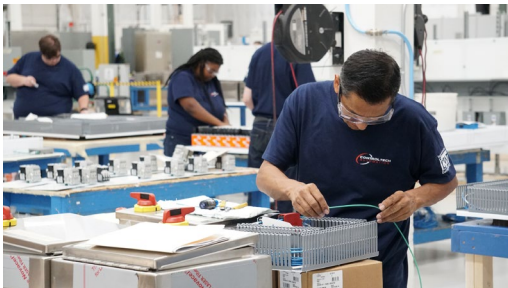
A technician assembles a control panel at ControlTech Automation's new manufacturing facility in Maryland Heights.
