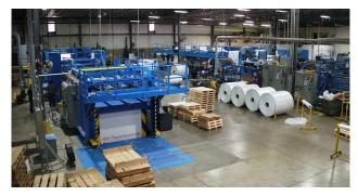
The SheetRunner is a dual-rotary sheeter, optimized for highvolume board production and designed for folding carton plants and commercial printers.
